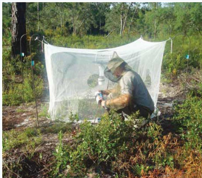
Figure 4: CDR David Hoel collecting mosquitoes from a light trap placed under a "failed" bed net (with holes) to measure the degree of mosquito ingress into the bed net. This project is a collaboration between CDC and USDA-CMAVE, Gainesville, FL.
