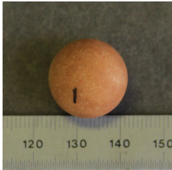
FIGURE 7. Spherical CompB Sample (mm Scale).
