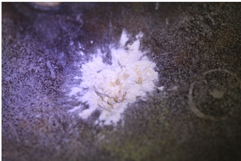
FIGURE 14. Impact Target With CompB Cylindrical Sample Debris.
