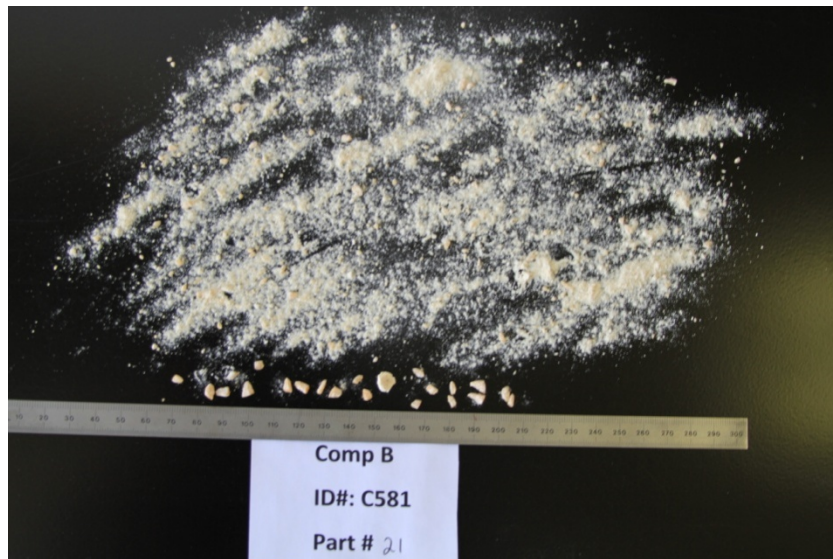
FIGURE 29. Spherical CompB Sample Impact Damaged at 370 ft/s.
