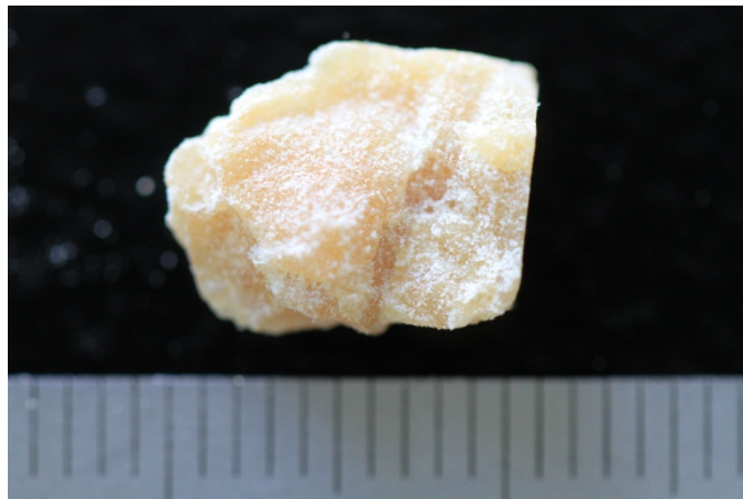
FIGURE 23. Fine CompB Coating Large Fragment (mm Scale).
