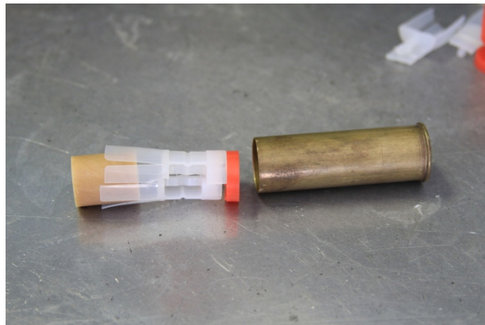
FIGURE 4. 18-mm Arrangement for the Cylindrical Samples.
