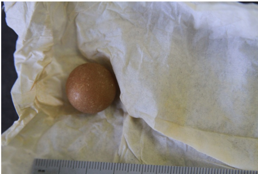
FIGURE 6. Residue From Spherical CompB Sample.
