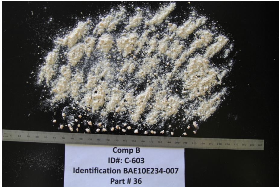
FIGURE 31. Spherical CompB Sample Impact Damaged at 435 ft/s.
