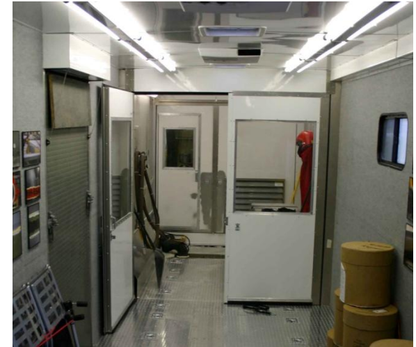
The mobile facility includes a fully enclosed blast room, media delivery system, material recovery system, and personal protective equipment
