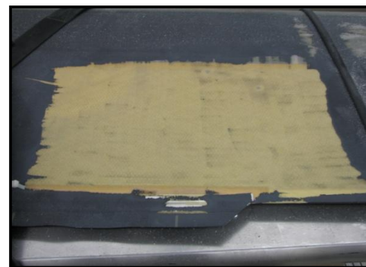
Coatings removed to fiberglass substrate at a rate of 34.4 ft 2 /hr (@ 32psi) with no substrate damage
