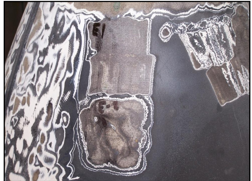
Coating removed from C-130 spinner cap at a rate of 10 ft 2 /hr with no visual damage to the substrate (fiberglass) or embedded electrical wires
