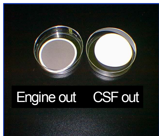
Figure 3. Effectiveness of a CSF in Reducing Total Particulate Mass.
