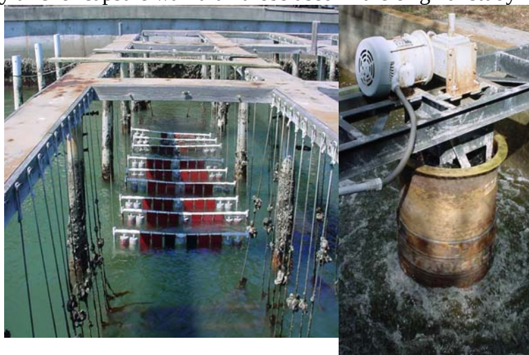
Figure 5. Florida test site. A) static panel exposure. B) dynamic panel exposure
