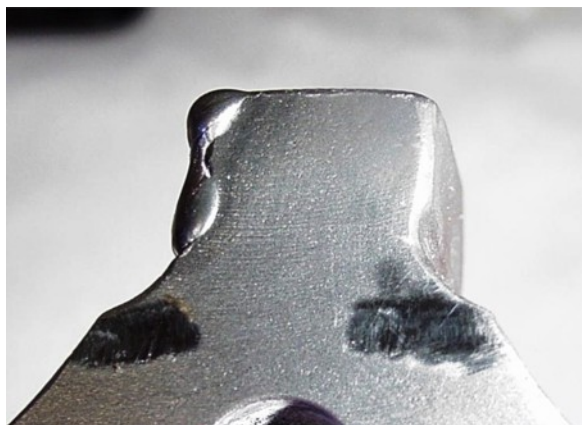
Figure 4-103 Excavate Damages Area
