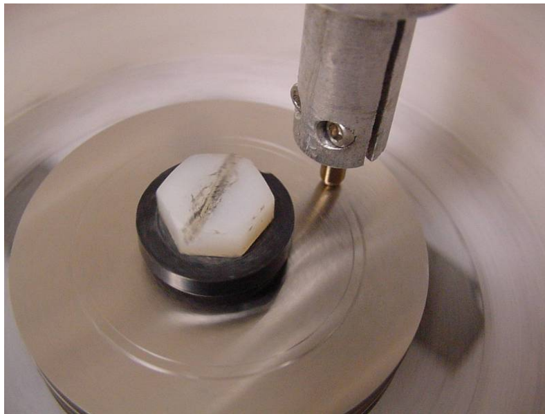
Figure 4-69 Running Pin/Disk Set-up Tests
