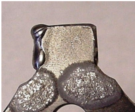
Figure 4-104 Repair Excavated Area
