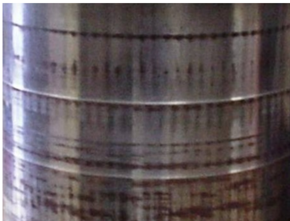
Figure 4-114 Worn Chrome Surface on Journal of TF39 Shaft
