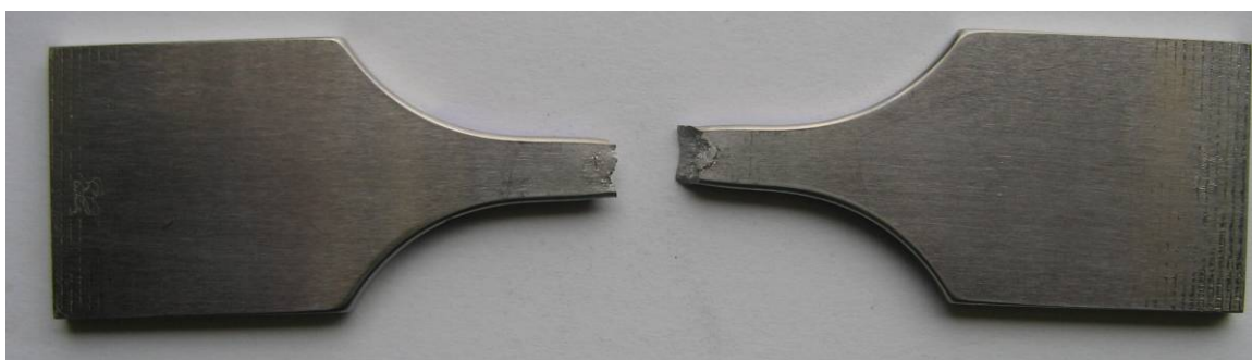
Figure 4-61 Typical Fracture of V4 Tensile Bar
