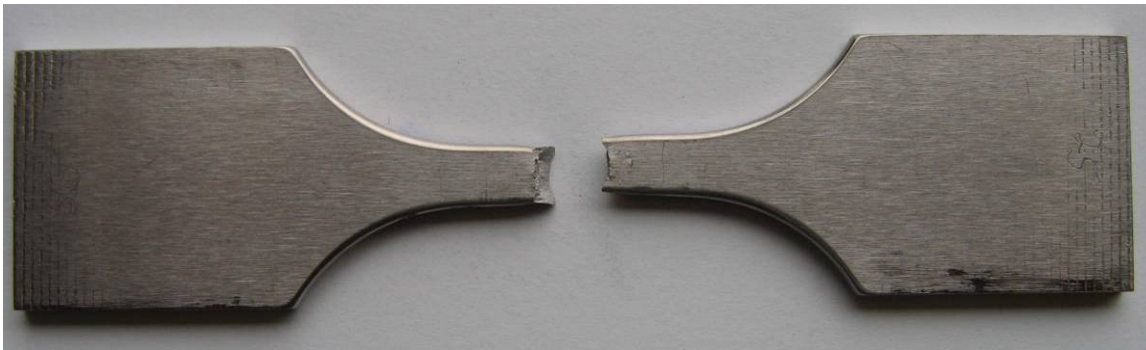
Figure 4-63 Typical Fracture of #32 with UIT Tensile Bar.
