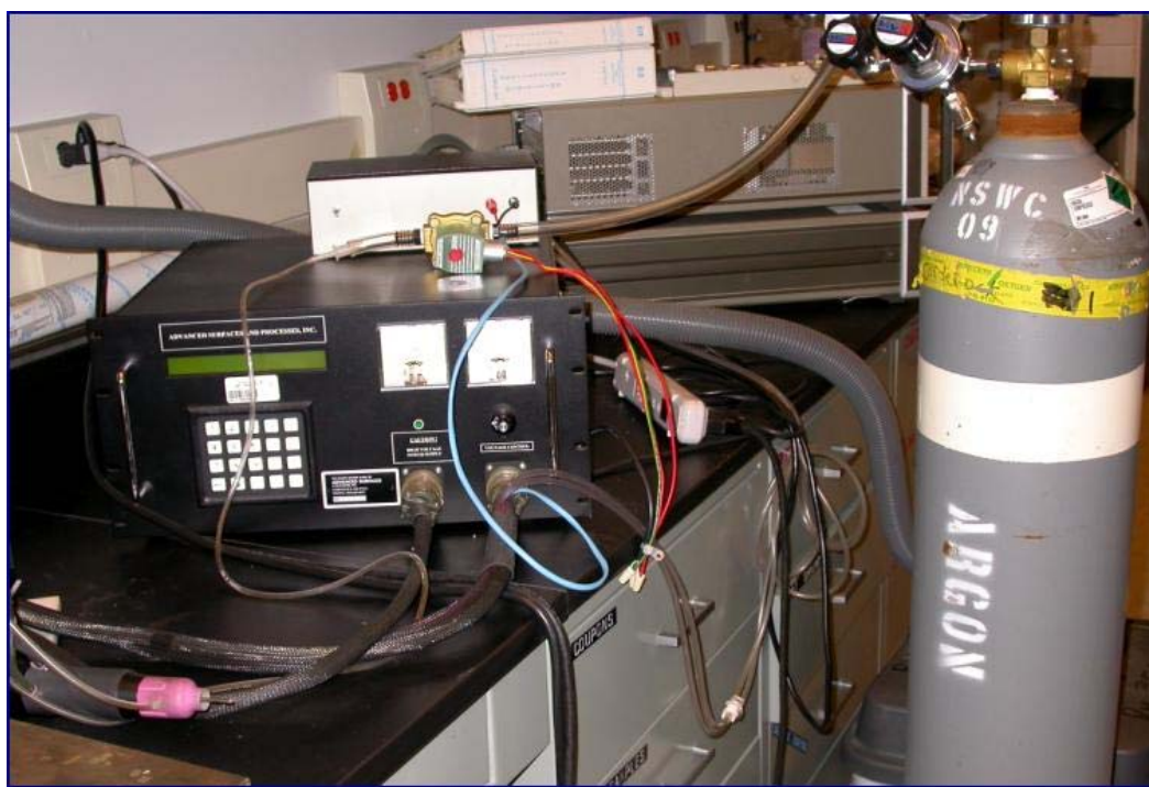
Figure 6-4 ESD Equipment Located at NSWCCD Used for Materials Studies
