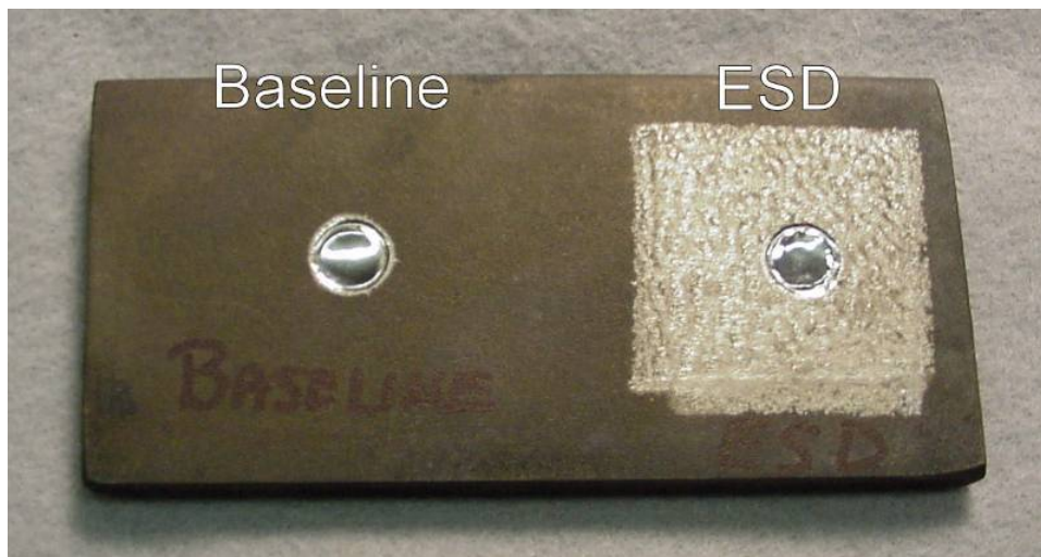
Figure 3-37 Residual Stress Coupon (Baseline and As Deposited ESD)
