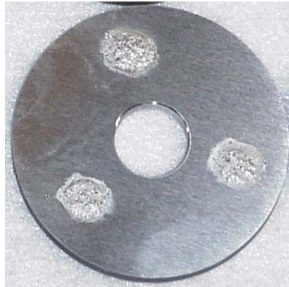
Figure 4-65 Pin-on-Disk Wear Test Specimen (Before Surface-finishing)
