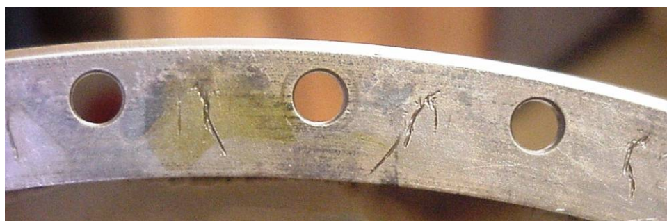
Figure 4-116 Hot Air Erosion on flange of TF39 Shaft
