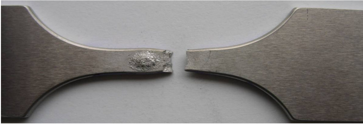
Figure 4-62 Typical Fracture of Bead-on-Plate Tensile Bar.
