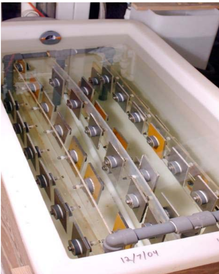
Figure 6-18 Crevice Corrosion Test Assemblies Immersed in Seawater
