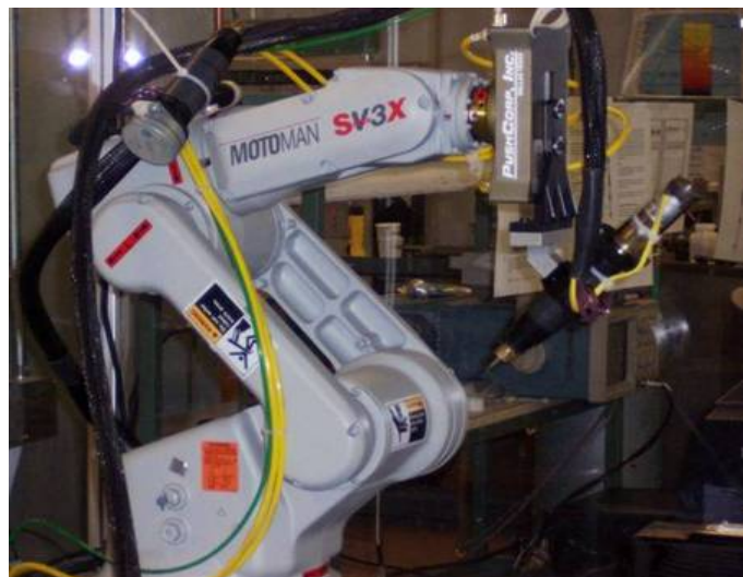
Figure 3-7 MOTOMAN SV3X Robot With PushCorp Pneumatic Load Control System
