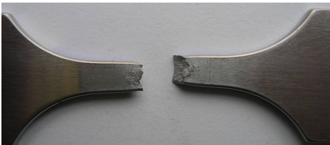
Figure 4-60 Typical Fracture of #32 Tensile Bar.
