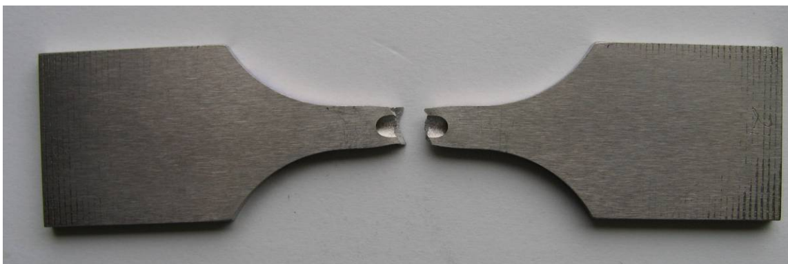
Figure 4-59 Typical Fracture of Baseline with Defect Tensile Bar.
