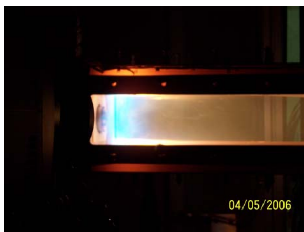
Figure 3.5.7-4. Photographs of Combustor Burning Heptane/Toluene at \Phi=1.1 : (top) no additive, (bottom) 1000 ppm.
