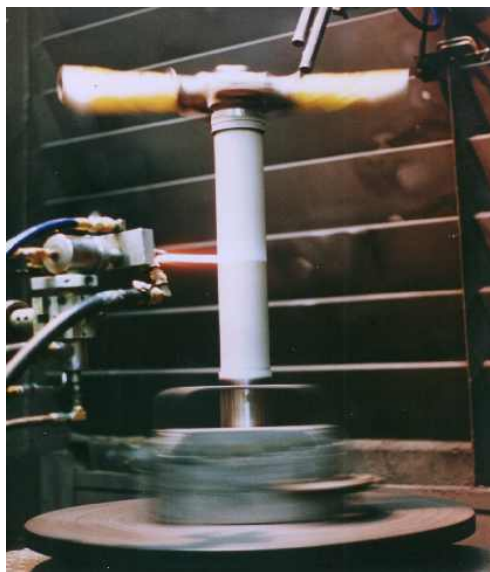
Figure 2. HVOF Spray of Landing Gear Inner Cylinder
