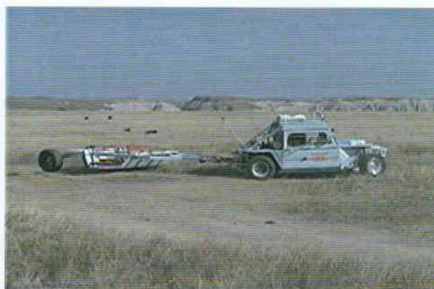
Figure 2. The MTADS survey system deployed with the pulsed induction array.
