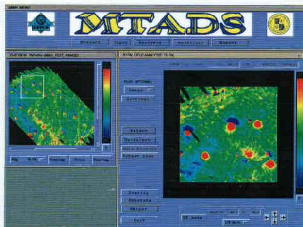
Figure 3. The MTADS data analysis system showing the site view and target analysis windows.
