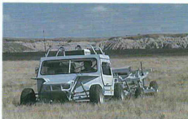
Figure 1. The MTADS Tow Vehicle surveying with the magnetometer array.
