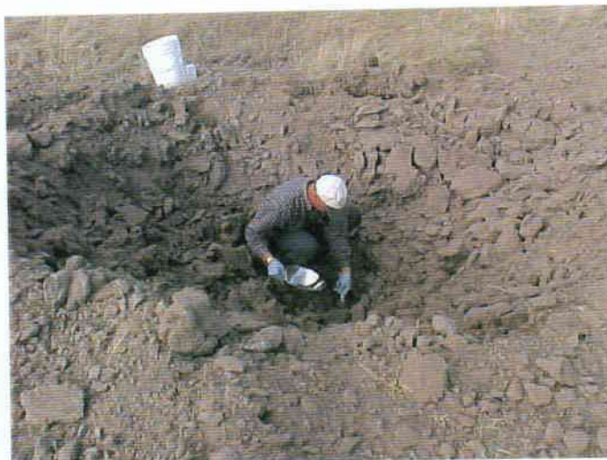
Figure 18. Soil samples were collected from several points within each detonation crater.
