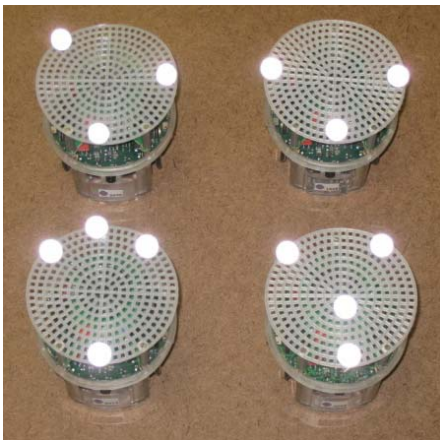
Figure 7: Optical Tracking Reflectors on E-puck Robots.
