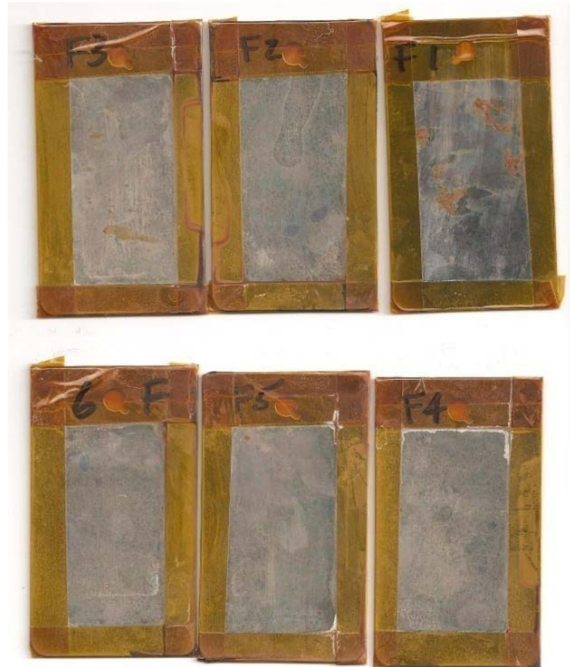
Corrosion Panels after 1000 hrs B-117 Exposure (Note: Panel 1 was exposed for only 24 hrs)
