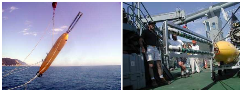
Fig. 1. On the left, the robot, Caribou , being lowered into the water off the coast of Elba. On the right is a close up of the 16-element dual line array used to receive the sonar signals. The green spheres are individual hydrophones.
