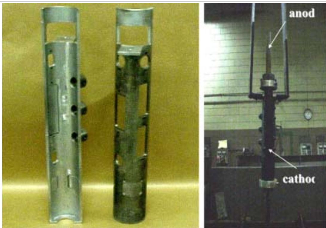
Figure 4-2 Hard chrome electroplating arrangement.
