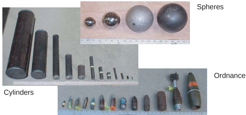
Figure 3. A variety of test objects were measured to investigate the capabilities of the GEM-3 and to provide a basis for analysis.
