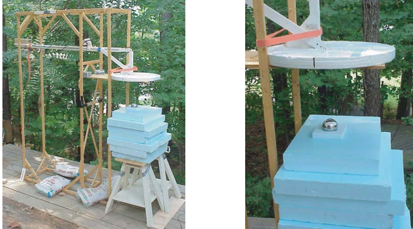
Figure 2. The GEM-3 instrument was set up to measure test objects under controlled conditions. This pictures shows a 3-inch diameter steel ball being tested.
