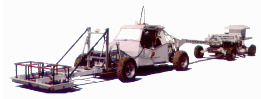
Figure 5: STOLS with front-mounted EM61 coils as deployed at JPG3.
