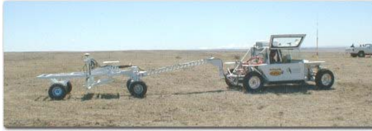
Figure 4: The MTADS vehicle and towed magnetometer platform developed by GEO-CENTERS for NRL in 1995.
