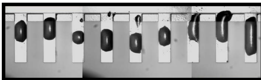
Fig. 2. Picture of ionic-liquid coated microcantilevers.
