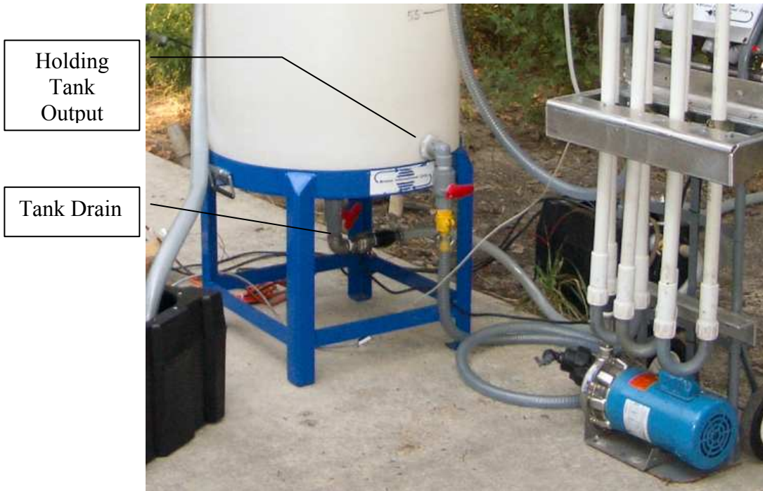
Figure 18: Bristol Holding Tank - Detail
