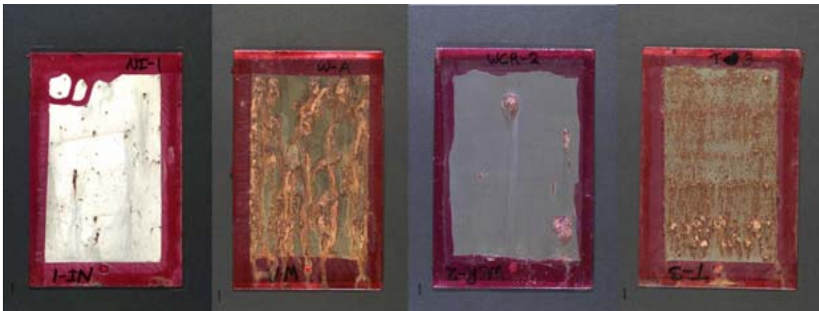
Figure 15. (Left to right) Comparison of 0.001"-Thick Electrodeposited Hard Nickel, HVOF WC/17Co, WC/10Co4Cr, and T800; After 8 Days of Exposure in the B117 Salt-Fog Cabinet.
