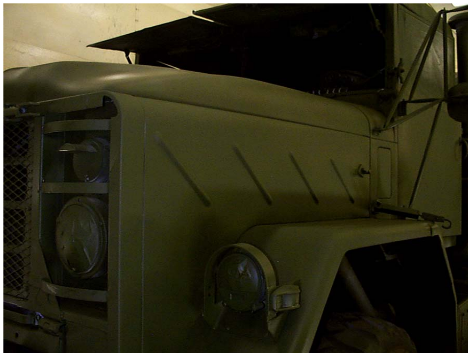
Figure 6 -- 5-Ton Truck after WD CARC Application at MCB
