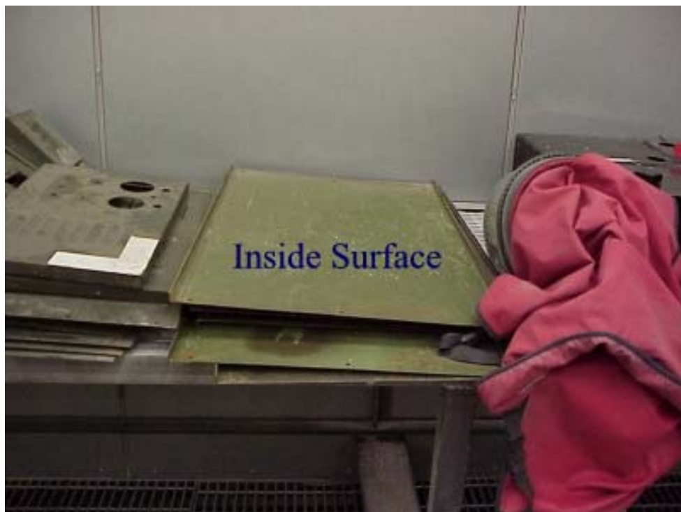
Figure 34 -- Covers Blasted in OO-ALC, Building 843 Blast Booth
