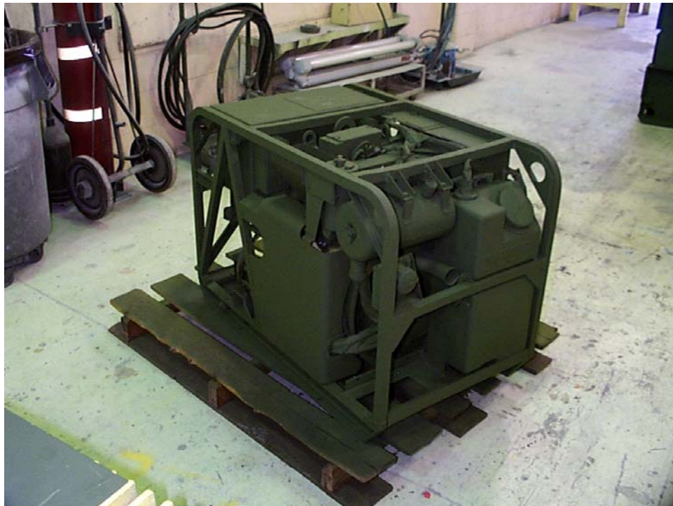
Figure 14 -- MEP-005A Generator after Application of WD CARC at Ogden ALC
