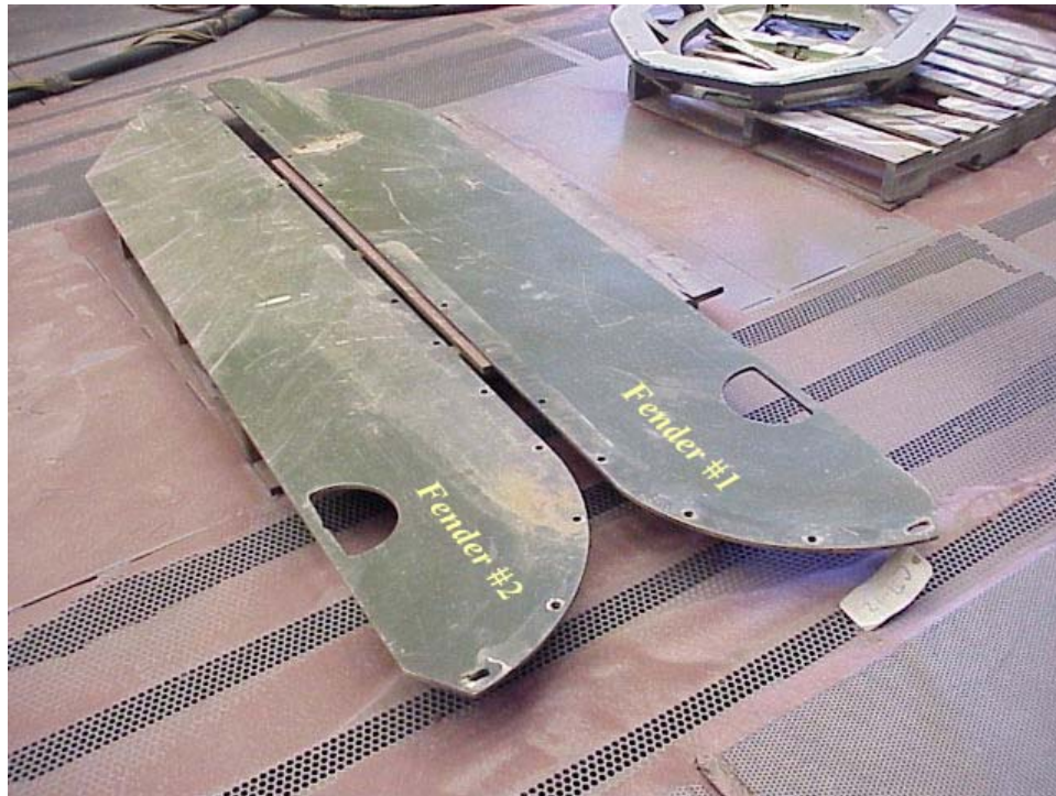
Figure 38 -- AAV Fenders Prior to Stripping with Garnet DMB at Albany MCLB
