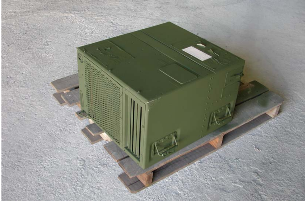
Figure 17 – 9000-BTU AC Unit before Application of WD CARC at Tobyhanna AD
