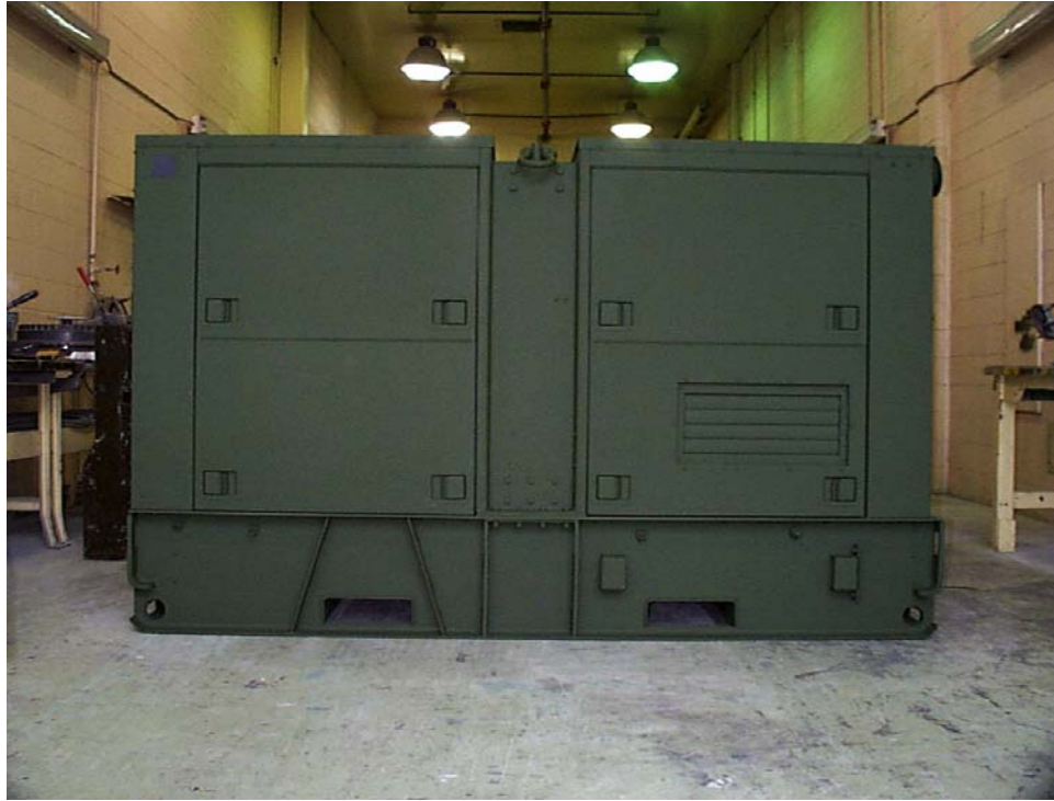
Figure 13 -- MEP-007B Generator after Application of WD CARC at Ogden ALC
