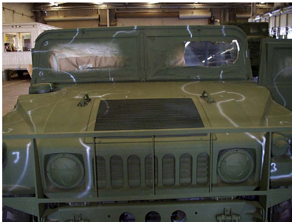
Figure 5 -- Vehicle 544264 (Front View) with Green WD CARC, Stenciled for Pattern at MCB
