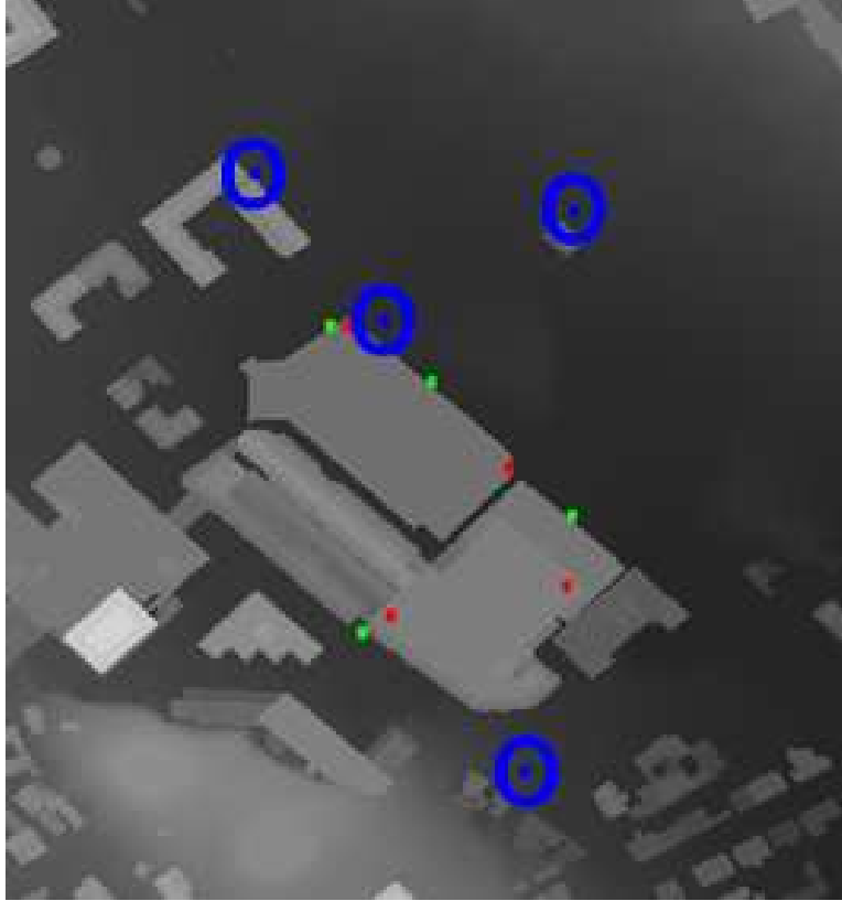
Figure 6. The solution of positions for four reconnaissance Soldiers to observe the targets (blue). The locations of the reconnaissance Soldiers were determined using the optimization based on minimizing ballistic threat while maximizing line-of-sight observation.
