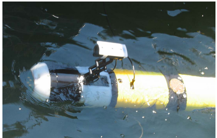
Figure 5. Photo of the extended periscope camera. The camera is mounted on a scissor jack assembly that permits it to be raised 9 inches above the vehicle. The camera is mounted at an angle of 5 degrees looking up. Camera electronics with recording system are housed forward of the camera.
