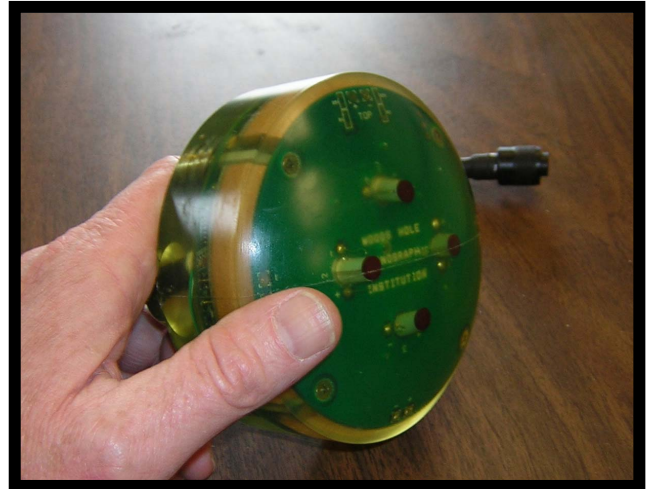
Figure 3 Photo of the USBL array showing the locations of the electronics, and acoustic receive array.
