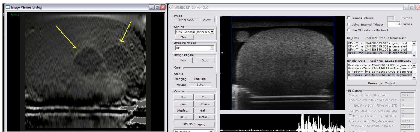
Figure 7: Elastogram and classic B-mode ultrasound for 3 stiff lesions inside prostate phantom Model 066 - TRUS probe imaging
