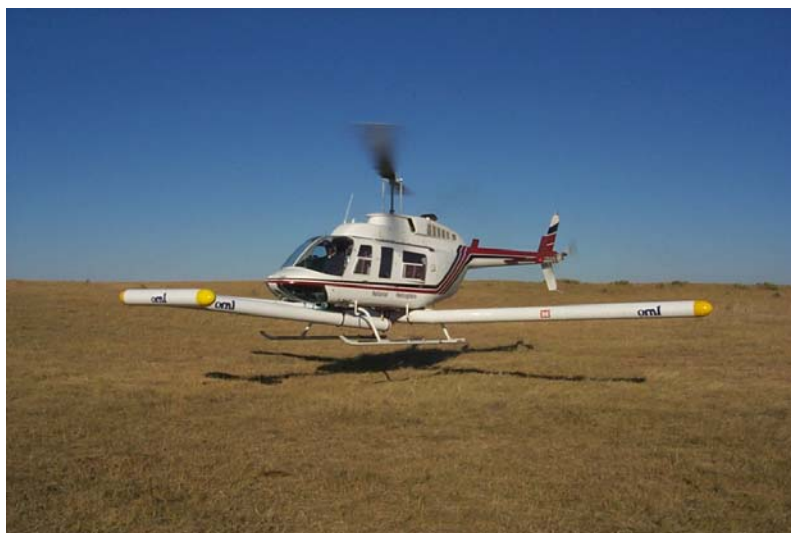
Figure 2.4 ORAGS-Hammerhead airborne magnetometer system used at Badlands Bombing Range in FY2000.
