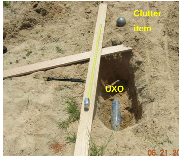
Figure 13. Hole dug in sand pit with 105 mm projectile placed horizontally at bottom and clutter item (shotput) on surface, with meter measure.
