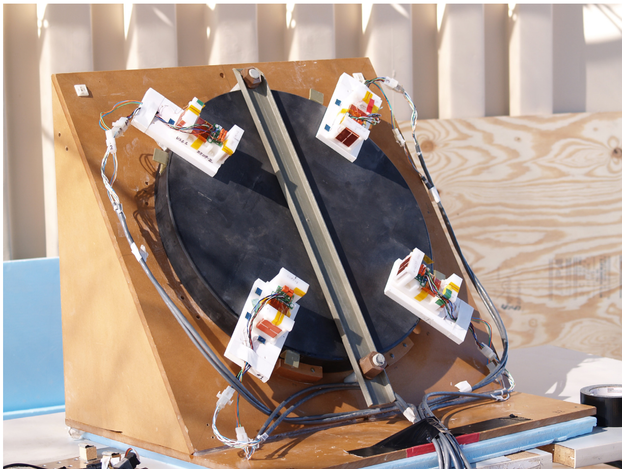
Figure 5.3.2.2. The magnetometer array mounted on the lectern (brown material) at a 57-degree inclination. The clamping bar and stops around the perimeter of the array prevented it from shifting while the array was manipulated for various experiments.
