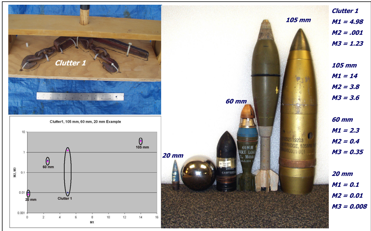
Figure 5.5.1.12. This figure shows inversions for M1, M2, and M3 for 20 mm, 60 mm, and 105 mm UXO items and for the clutter item shown. For the UXO items the calculated M2 and M3 are close together which is an indication of rotational symmetry and therefore likely UXO. For the clutter item no two of the three M's are close together, indicating a non-symmetric shape.
