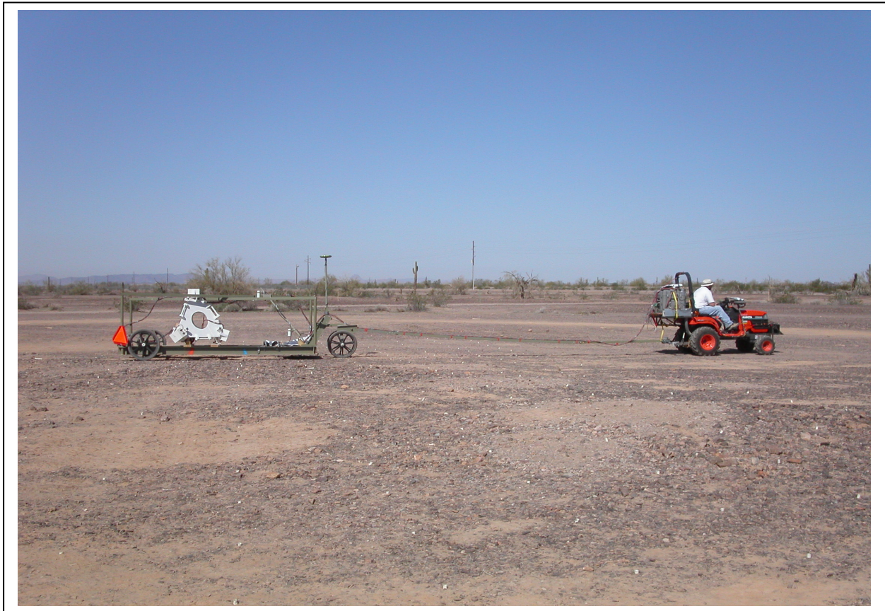
Figure 5.1.3.1. This figure shows the TMGS in its original tetrahedral configuration at YPG. The tow bar is 7 m long to reduce the effect of the tractor signature on the data.
