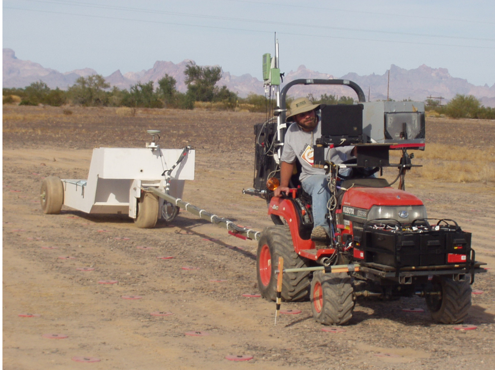
Figure 5.3.2.16. The TMGS in operation over the Calibration Grid. The operator used a simple outrigger pointer to guide the tractor between large red disks that marked the corners of individual cells.
