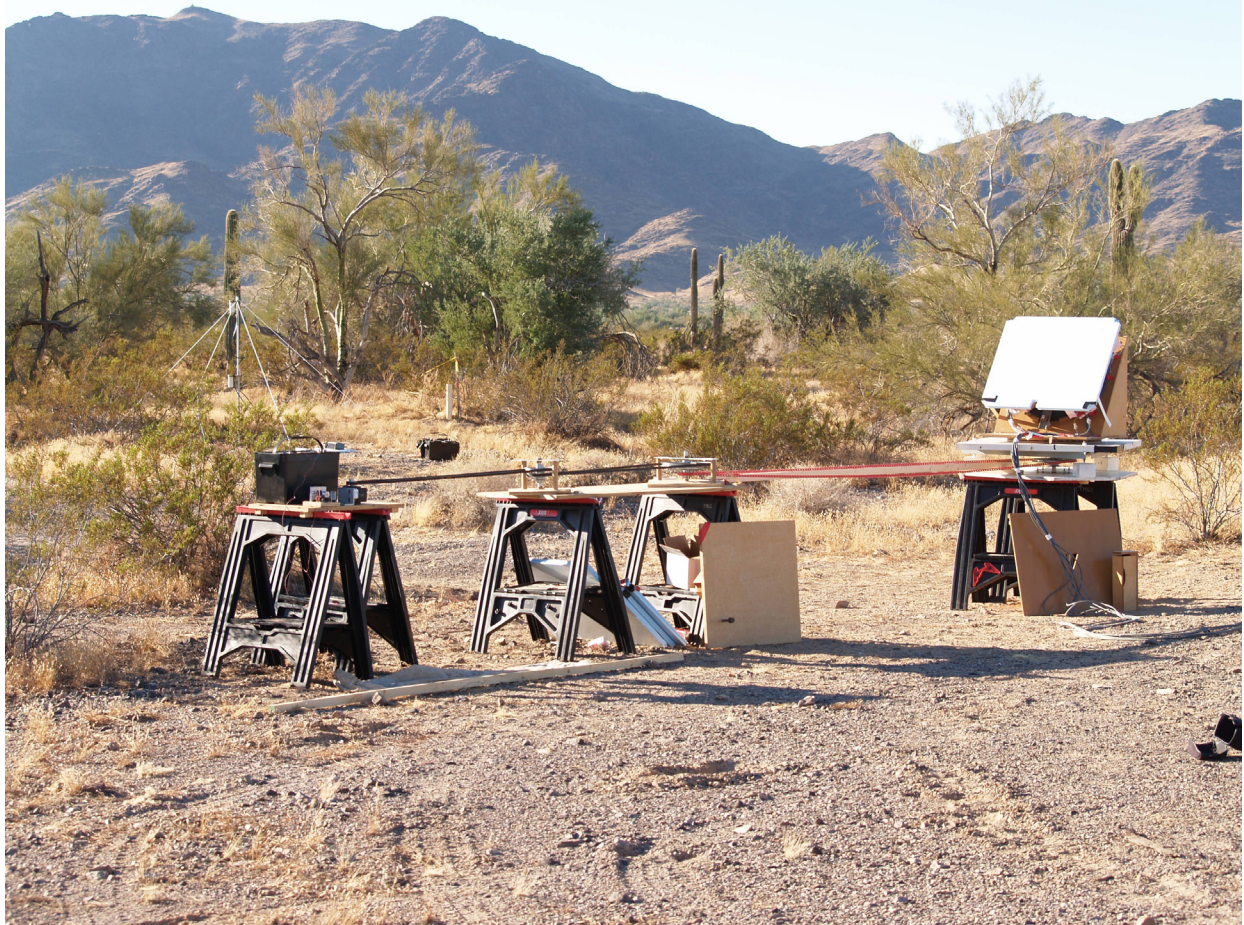
Figure 5.3.2.1. The spin calibration apparatus set up at a magnetically clean location for a calibration run. The electric motor drive assembly (left) transmits power through a set of tandem pulleys (center) to the rotating platen on the turntable assembly (right). The magnetometer array is mounted on a lectern which rests on the turntable platen. The array is shielded from direct sunlight in order to minimize large, rapid temperature variations.
