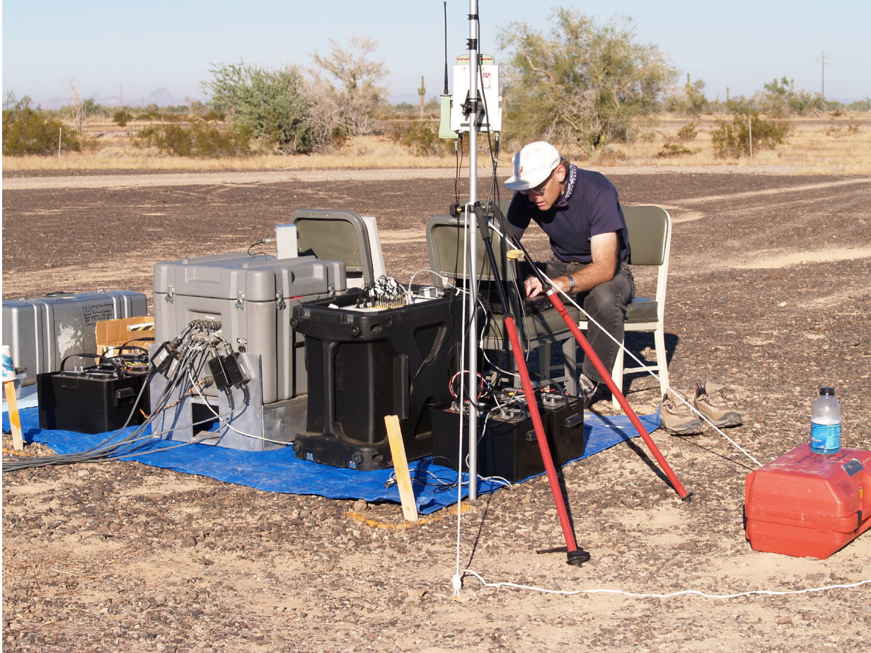
Figure 5.3.2.3. The TMGS data acquisition system was stationed about 10 m away from the magnetometer array. The magnetometer interface unit (square grey case on left) and the NI computer (tall black case) are flanked by lead acid batteries. The GPS receiver (top center, on the pole) supplied PPS timing pulses.
