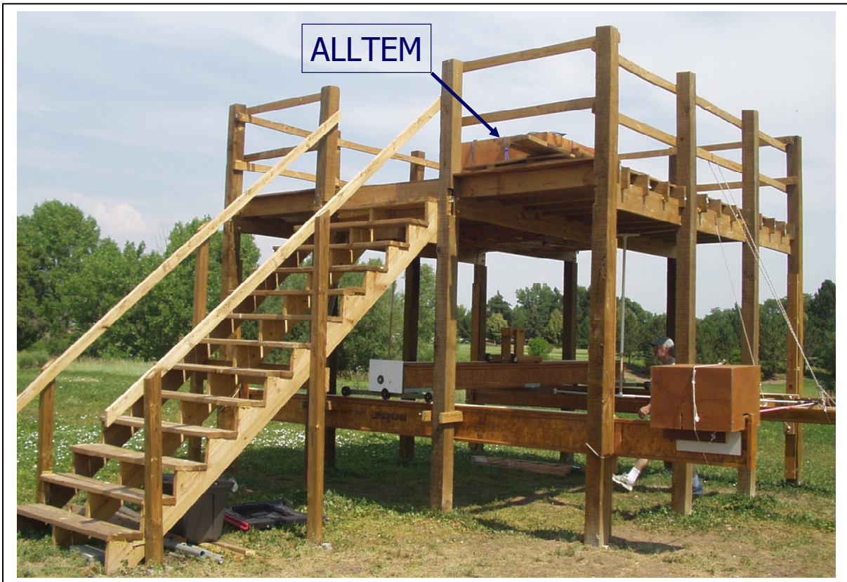
Figure 5.5.1. The ALLTEM cube is mounted under a cover on the test stand deck. Ordnance and clutter items are moved underneath the deck by computer-controlled stepper motors. Positions are measured by a combination of a string potentiometer and lasers and are accurate to within +/- 3 mm.
