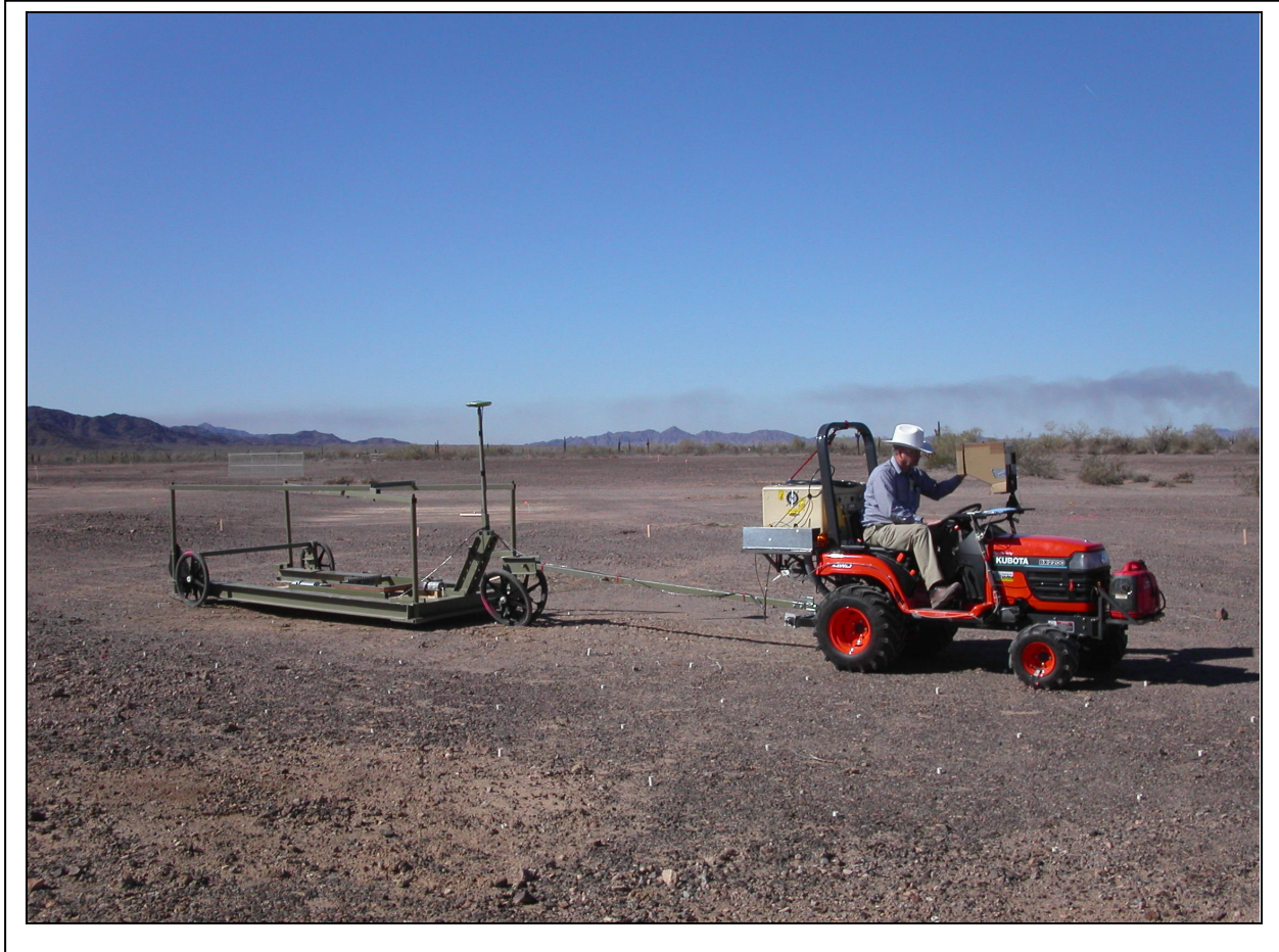
Figure 5.1.2.1.1. This photograph shows the VETEM system in operation at the YPG in 2003. The sub-compact tractor is advantageous because it is designed to operate at steady speeds.
