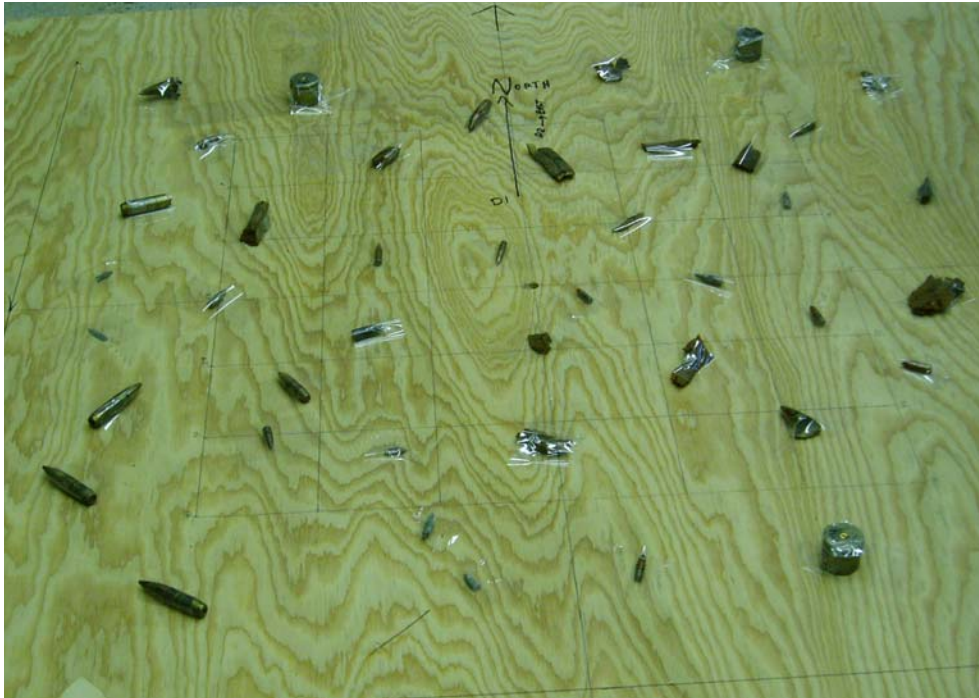
Figure 76. Sparse clutter example used in measurements, on 10 cm grid
