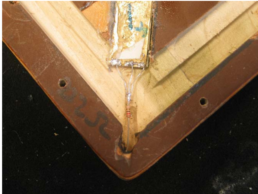
Figure 166 Termination of the antenna with a 120 \Omega lump resistances.
