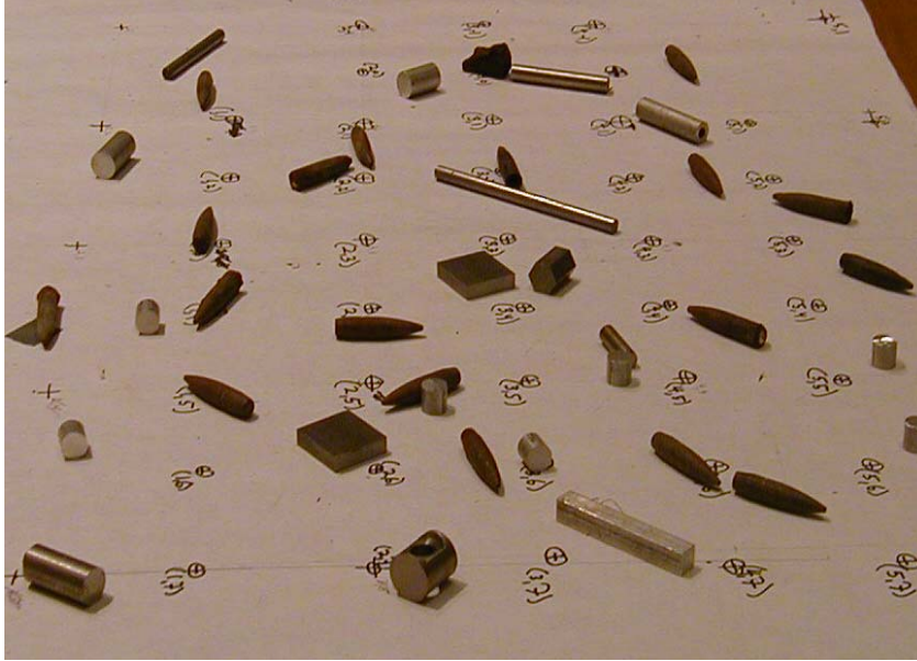
Figure 70. A sparse distribution of clutter items, some collected from firing ranges, relative to 10 cm spacing of grid marks.
