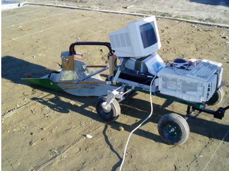
Figure 147. GPR cart with antenna pulled behind.
