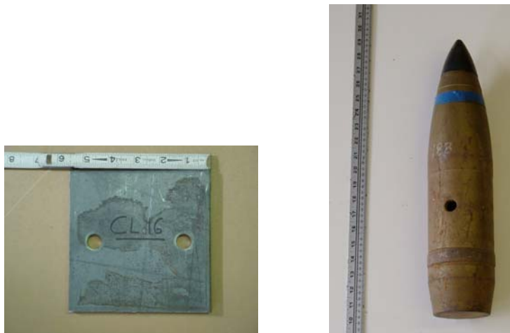
Figure 35. Left: 14 cm square clutter item placed 5 cm above and slightly offset from the approx 43 cm long UXO on the right.
