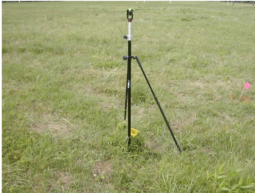
Figure 6 Reflector mounted on bipod setup on a known point. This instrument is used to confirm the position where the theodolite is setup.
