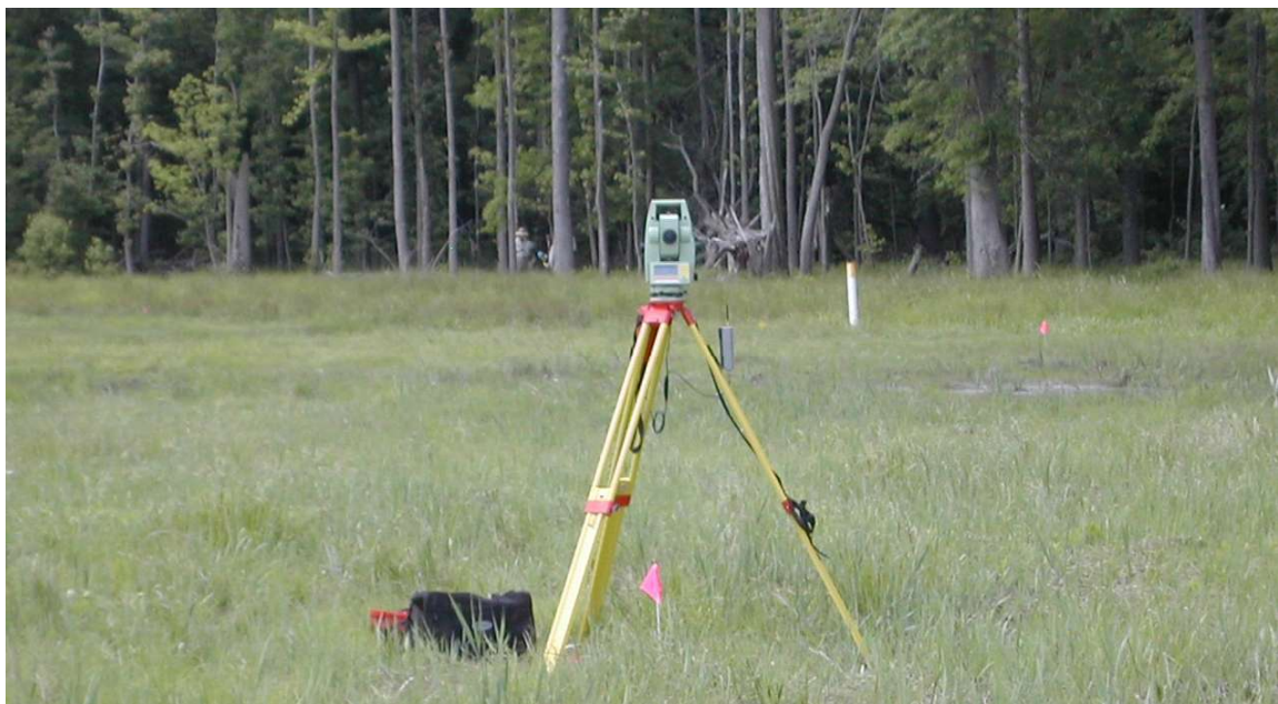
Figure 8 RTS shooting into wooded area from Theodolite Station 10D. The butt of the felled tree can be seen just to the right of the theodolite.
