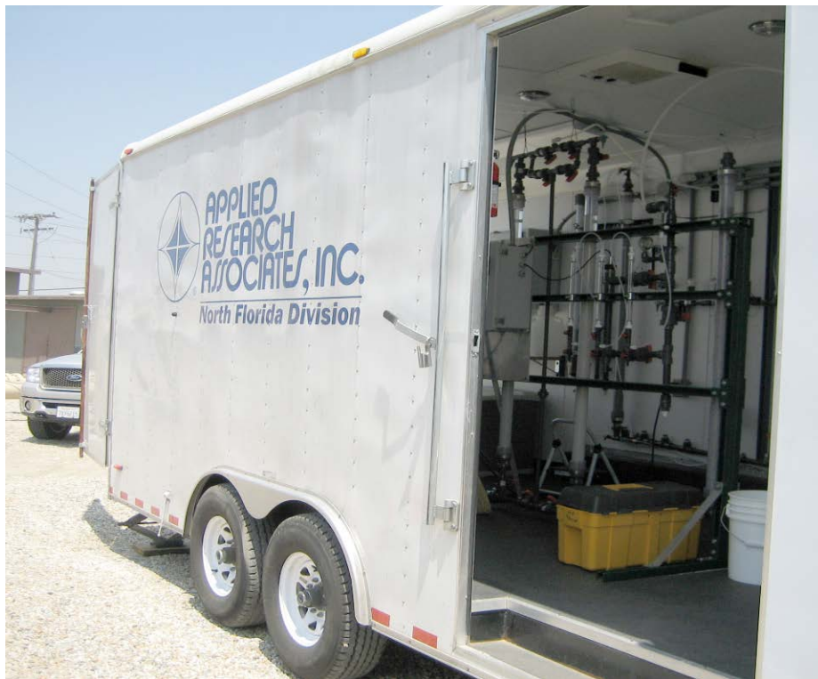
ARA demonstration trailer containing ion exchange equipment at well-site F-17 in Fontana, CA
