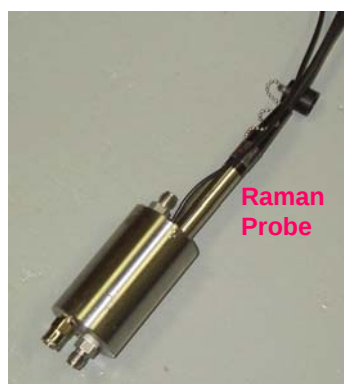
Figure 6. Fluidics unit with Raman probe and electrical cable.
