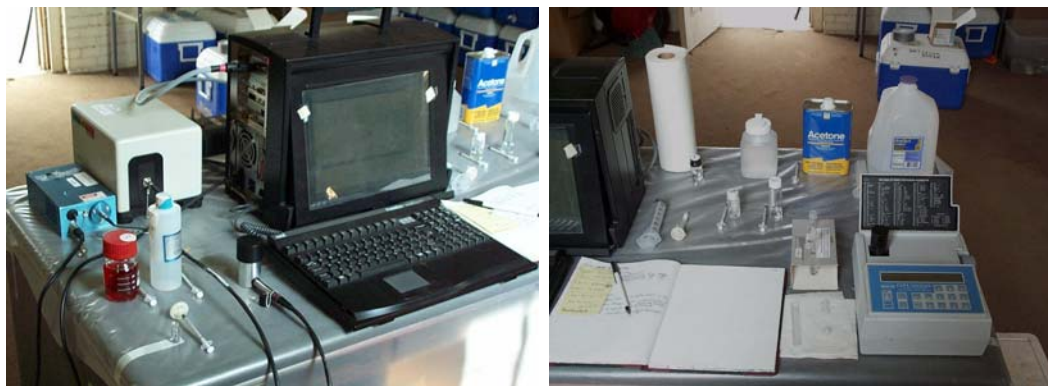
Figure 12. SERS (left) and colorimetry (right) methods set up on a desk at ALAAP.
