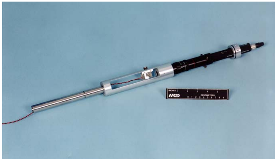
Figure 18. . Photograph of downhole video imaging system probe. Soil in contact with the sapphire window is illuminated with scattered light from white LEDs. The soil is imaged through a lens system coupled to a color CCD camera. The video signal is returned to the surface where it can be viewed in real-time and recorded using a video recorder or stored digitally.
