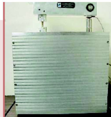
Side view of RSL™ computer controlled Type 1c test frame.
