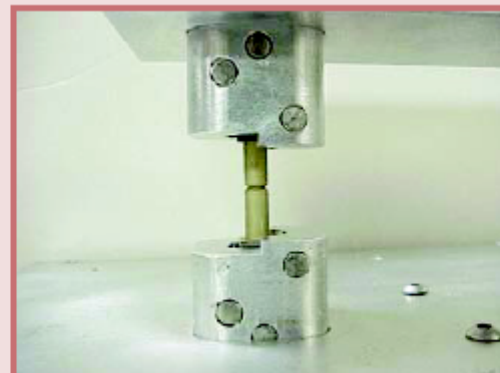
Type 1c Notched Round Bar plated specimen set into adaptor fixture for 24-hour RSL™ Accelerated Hydrogen Embrittlement Test.
