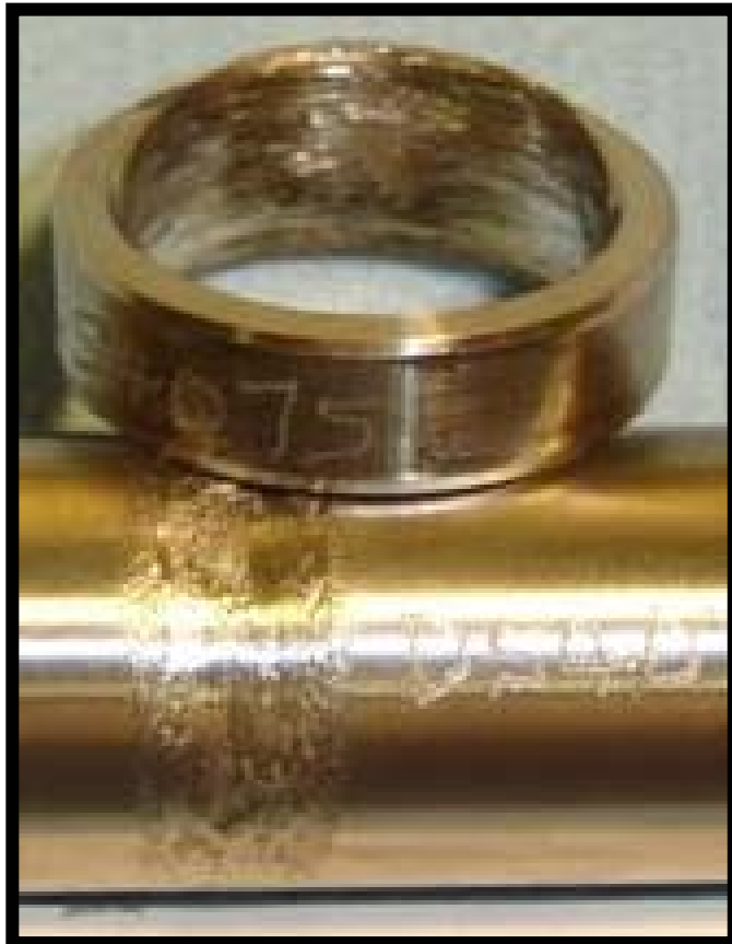
CW Nitronic 60 Bushing; MP 35N Pin 1850 cycles total 250 cycles at 10,000 lbs
