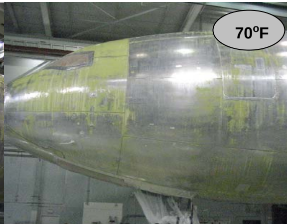
Alkaline cleaned 26 hours after 3 rd application
