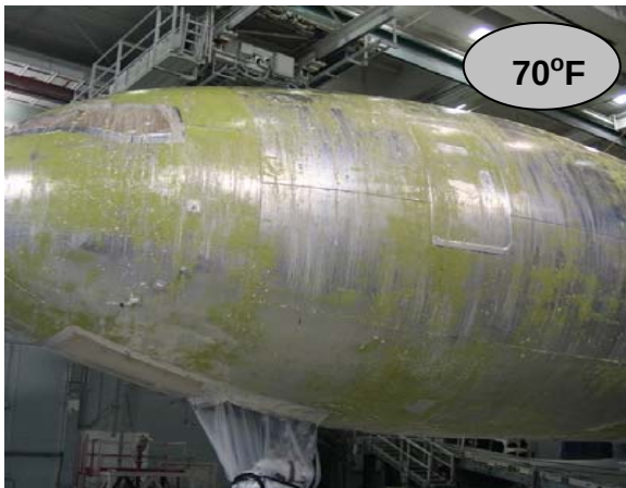
Squeegee after 2 nd full application coat
