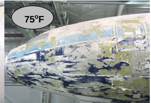
1 st Strip coat & 1.5 hours dwell
