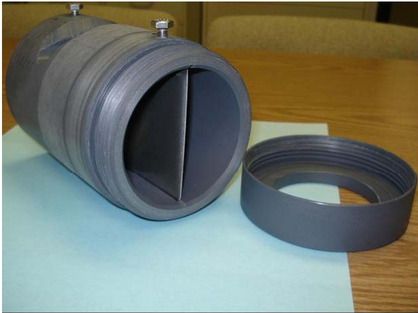
Hull Cell Test Panel Inserted In Plastic Tube
