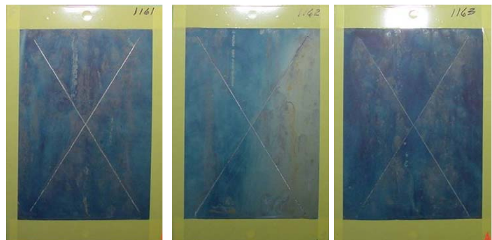
LHE Zinc-Nickel Plating – 1000 Hrs. ASTM B 117 Salt Spray Exposure
