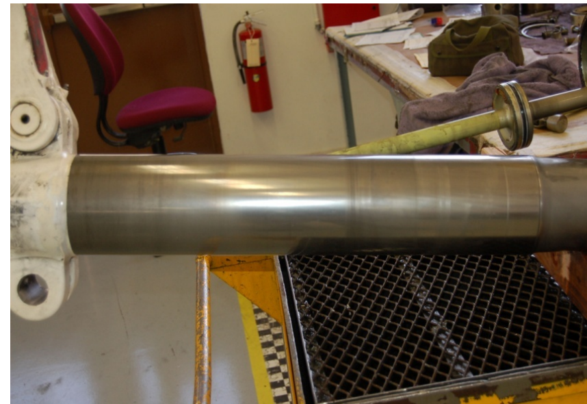
HVOF coated piston during disassembly
