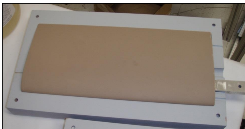
Figure 9: Completed flexible propulsor inside the open mold after curing.
