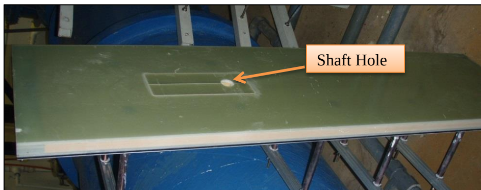
Figure 6: The grounding board of water channel prevents free-surface interaction during the tests.
