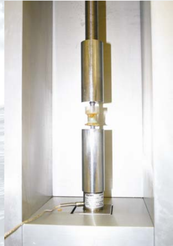
Round Bar Test in Progress
