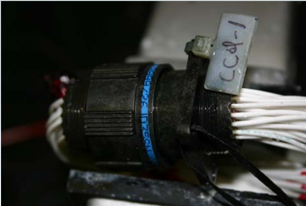
PEEK W/ Cadmium Plating
