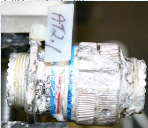
6061 Aluminum W/ Alumiplate Coating With TCP 25% dilution
