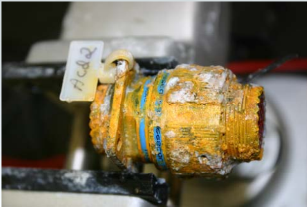
Cadmium plated 6061T6 Aluminum
