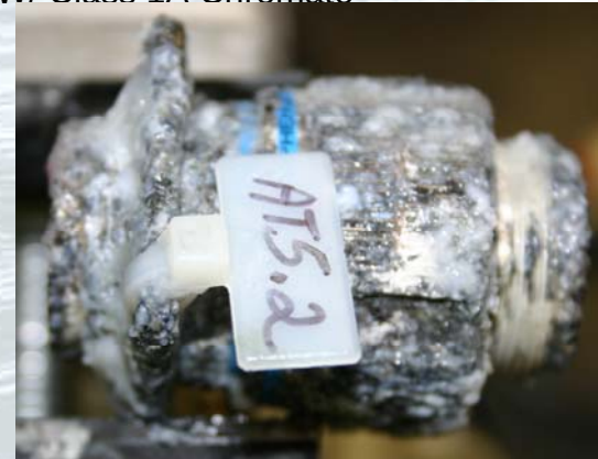
6061 Aluminum with Alumiplate coating W/ TCP 50% dilution
