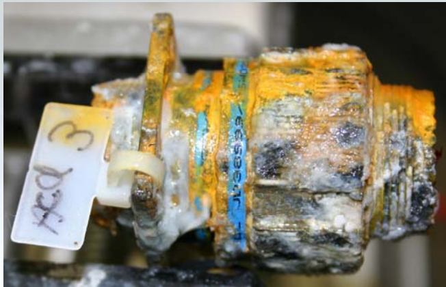
6061 Aluminum with OD Cadmium Plating
