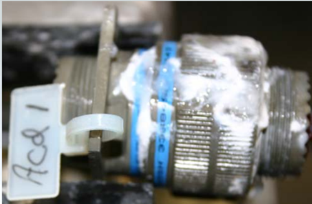
6061 Aluminum Connector W/OD Cadmium Plating
