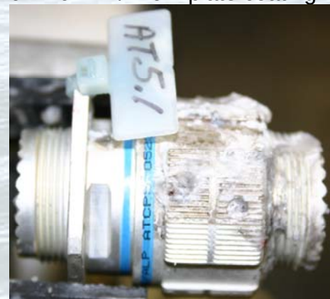
6061 Aluminum with Alumiplate coating and 50% TCP Dilution
