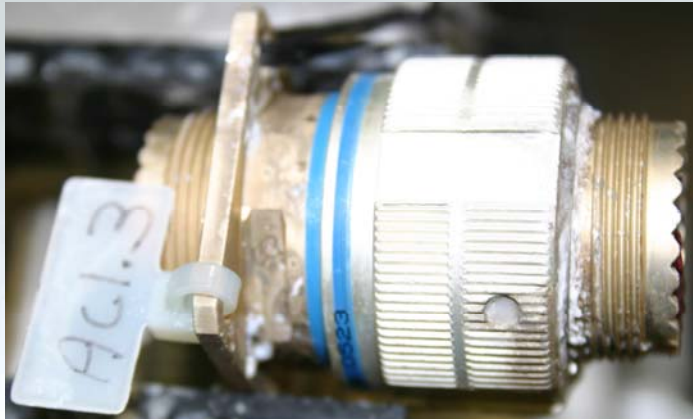
6061 Aluminum W/ Alumiplate coating coating Class 1A Chromate
