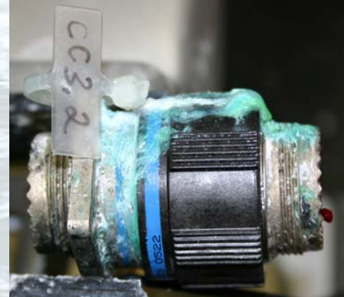
PEEK W/ Alumiplate & Class III Chromate
