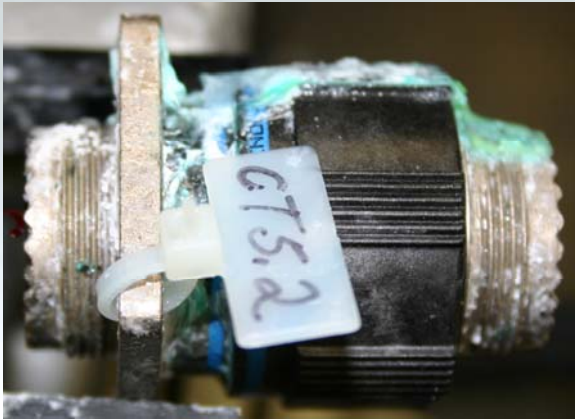
PEEK W/ Alumiplate coating & TCP 50% Dilution
