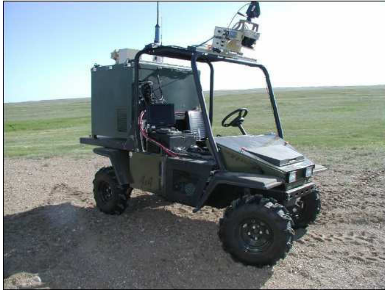
Figure 1: One of two Koyker Raptors used in the DRDC demonstrations. Each Raptor used one or more roof mounted SICK laser scanners, Digiclops stereo cameras, DGPS positioning, 3DMG inertial measurement units, and wireless mesh networking.
