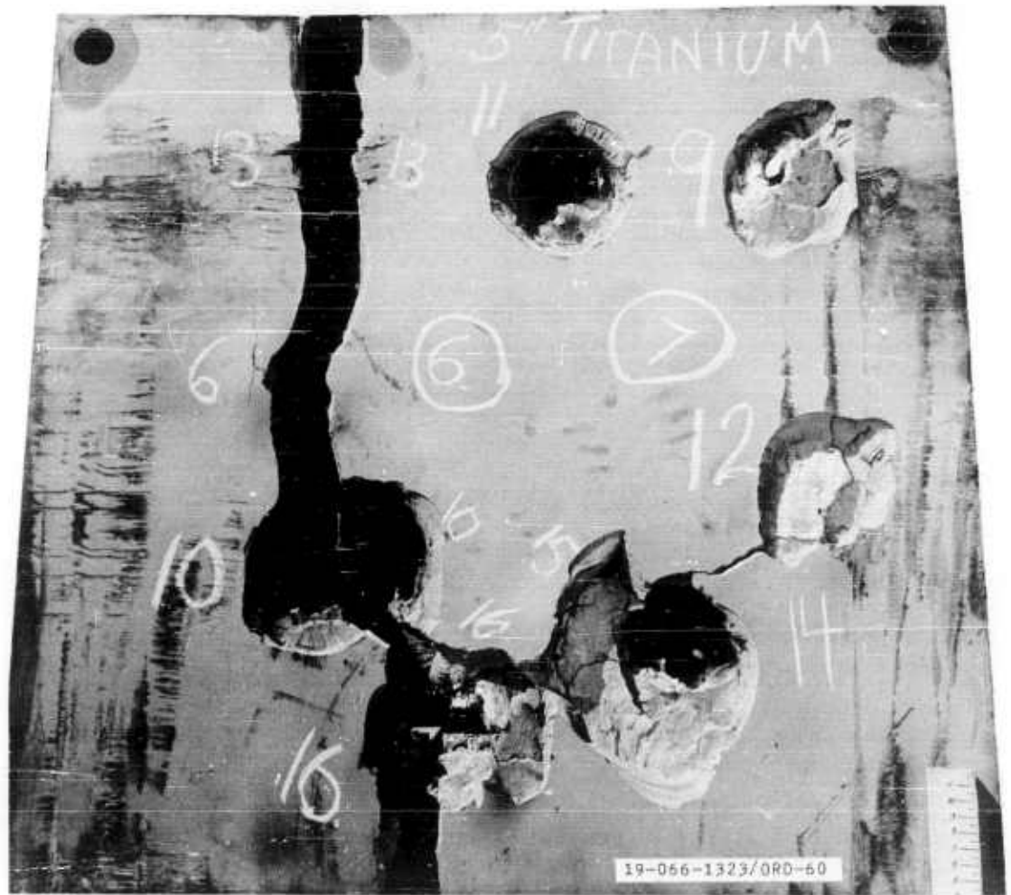
Figure 2 (U). TITANIUM ALLOY (6Al-4V) ANNEALED) 5-INCH-THICK PLATE AFTER ATTACK BY 90MM AP M318 PROJECTILE.(U)
