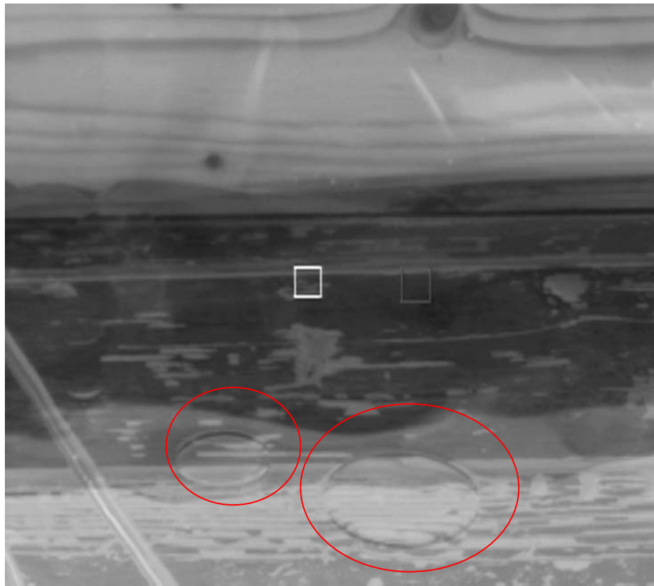
Figure 6. Picture of the water surface after contamination. Red circles show contaminant aggregation moving on water.
