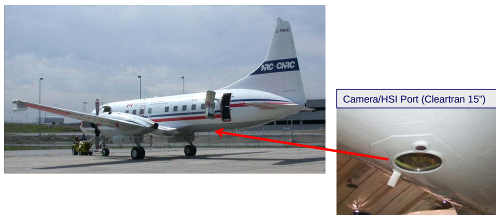
Figure 3: Convair aircraft showing the window mounted in the bottom of the plane to allow nadir measurements by the AIRIS sensor.
