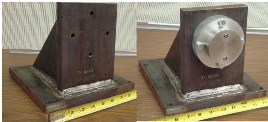
Figure 7.15. Machined and welded target fixture with and without the target assembly mounted
