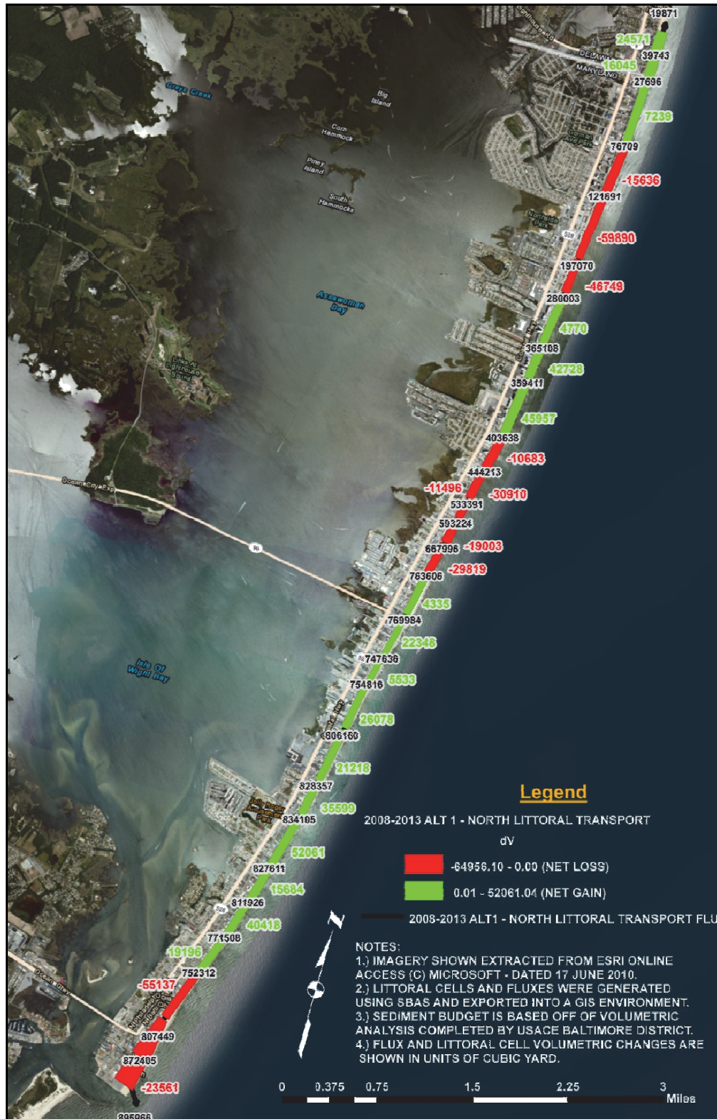
Figure 3. Atlantic Coast of Maryland sediment budget, Alternative 1, developed for the sediment budget update. May 2008–May 2013 epoch. North littoral transport.
