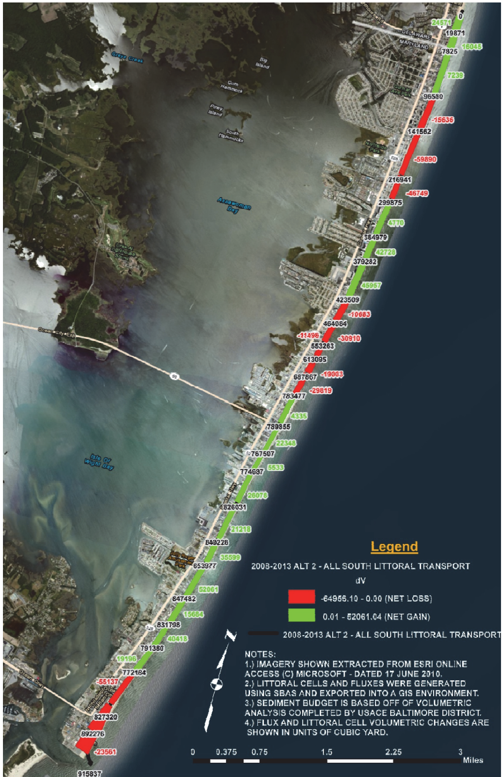
Figure 4. Atlantic Coast of Maryland sediment budget, Alternative 2, developed for the sediment budget update. May 2008–May 2013 epoch. All south littoral transport.
