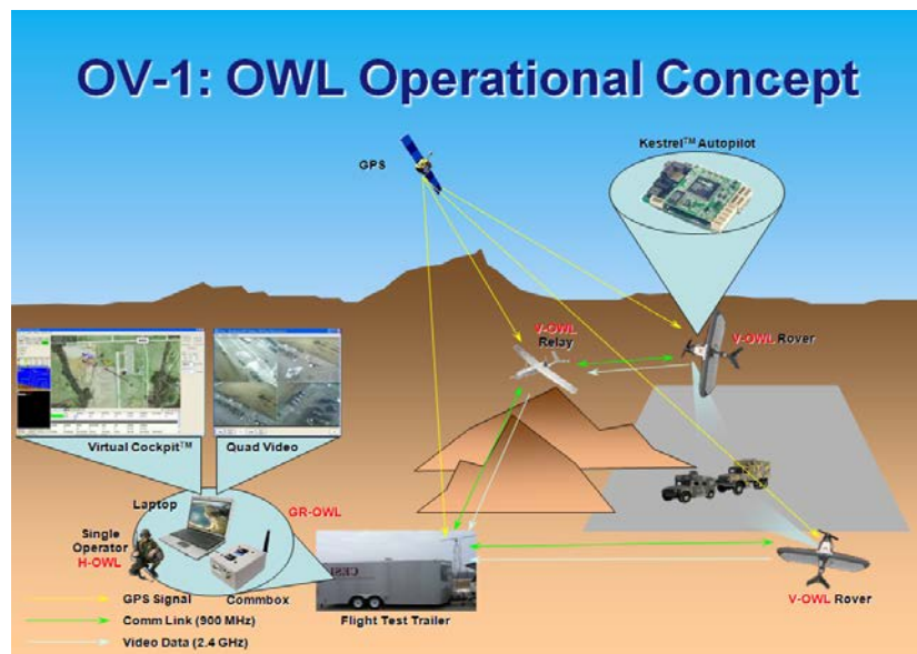
Figure 3. OV-1 of Seibert et al. Rover Relay System Concept [6, p. 24]
