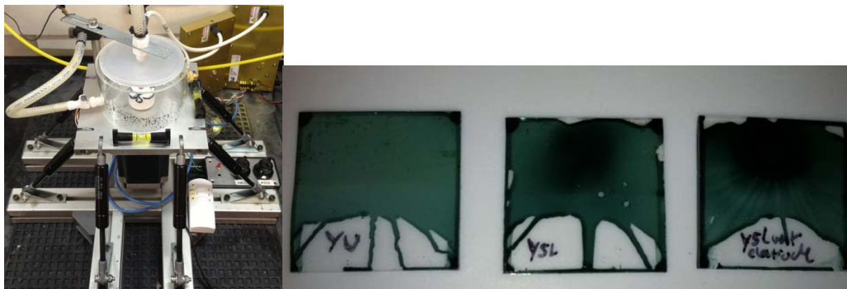
Figure 3. An image of the experimental apparatus constructed to produce OEOM films subjected to SPARC processing and a series of films the resulted from initial trials: (left), under standard SPARC conditions (middle) and under longer exposure to the corona discharge with a patterned ground electrode (right).
