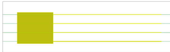
Figure 9. Top electrode configuration over optical waveguides
