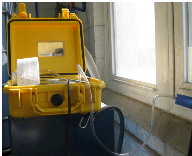
Figure 3: Example Pressure Transducer Installation
