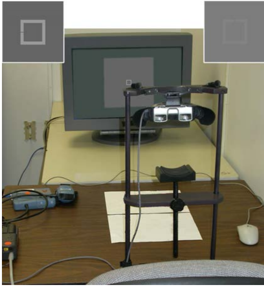
Figure 1: The experimental scene, consisting of the chin rest and monitor, with the Glasstron positioned for testing. This image corresponds to the viewing condition “Glasstron Through.” Modified Landolt-C stimuli are shown (upper left: contrast=0.2, gap=2 pix, open left; upper right: contrast=0.025, gap=5 pix, open up).
