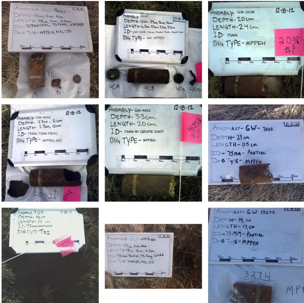
Figure 5-3. Recovered UXO from this demonstration
