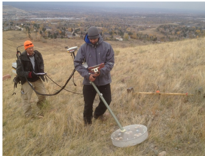
Figure 4-4. MPV cued data collection at Camp George West. The location beacon used for local positioning during cued operation can be seen on the right side of the photograph.
