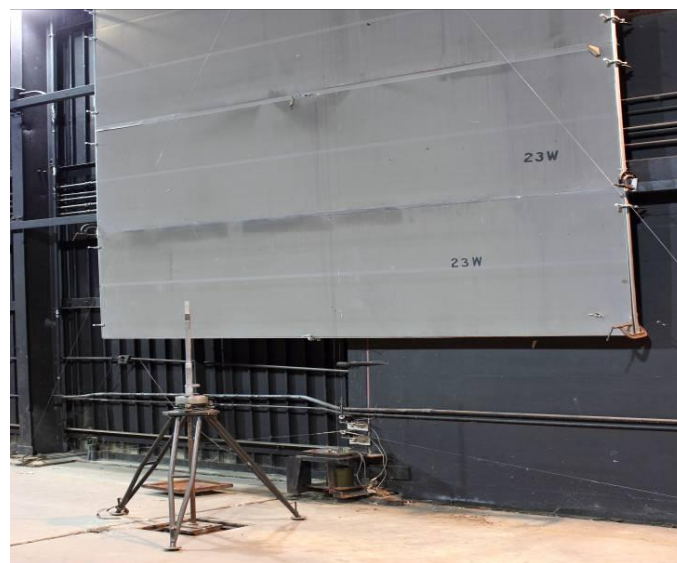
Figure 10. Lower section of elevation rod positioned over benchmark.
