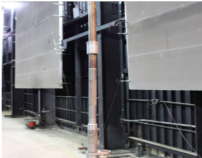
Figure 12. Micrometer barrel used to set the height of the elevation rod for each station.
