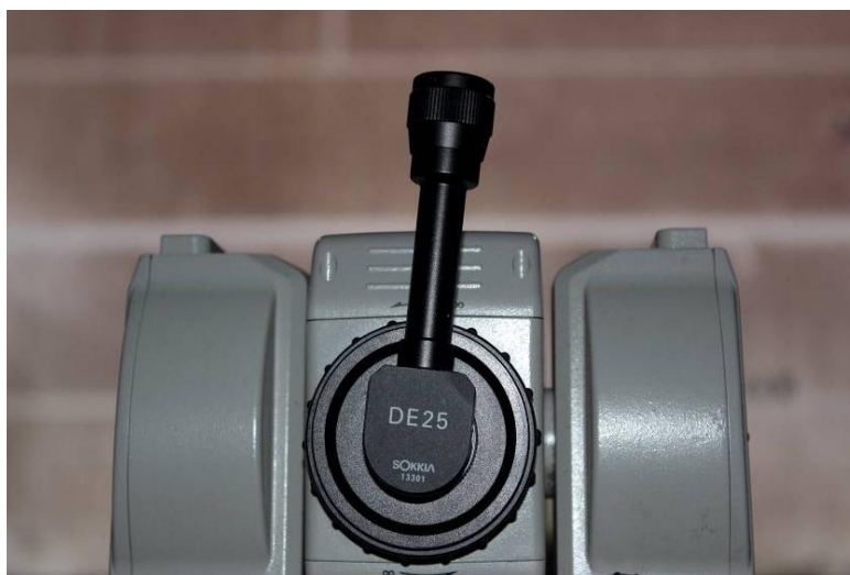
Figure 16. 90° elbow scope attached to theodolite head used to check the survey of the (pit) bead (spark side).
